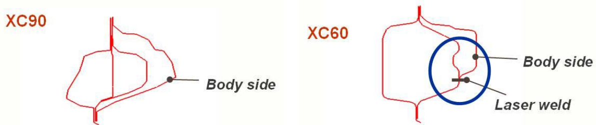
Figure 12. The solution with a "reduced body side" for the Volvo XC60 which means a weight saving of 1.5 kilograms in comparison to the XC90 design.
