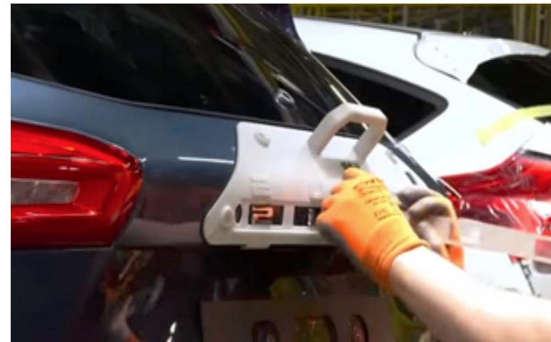
Guiding Jig for the Final Assembly Shop
