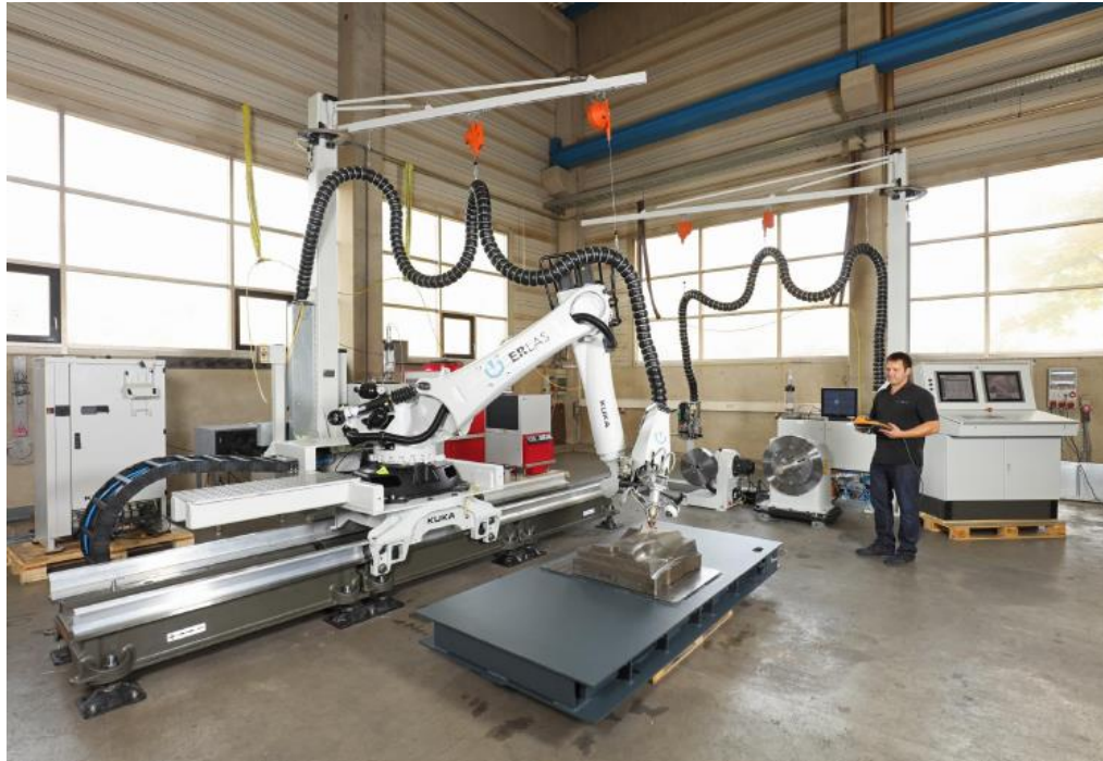
Laser processing with the combitool ERLAS HardClad™
